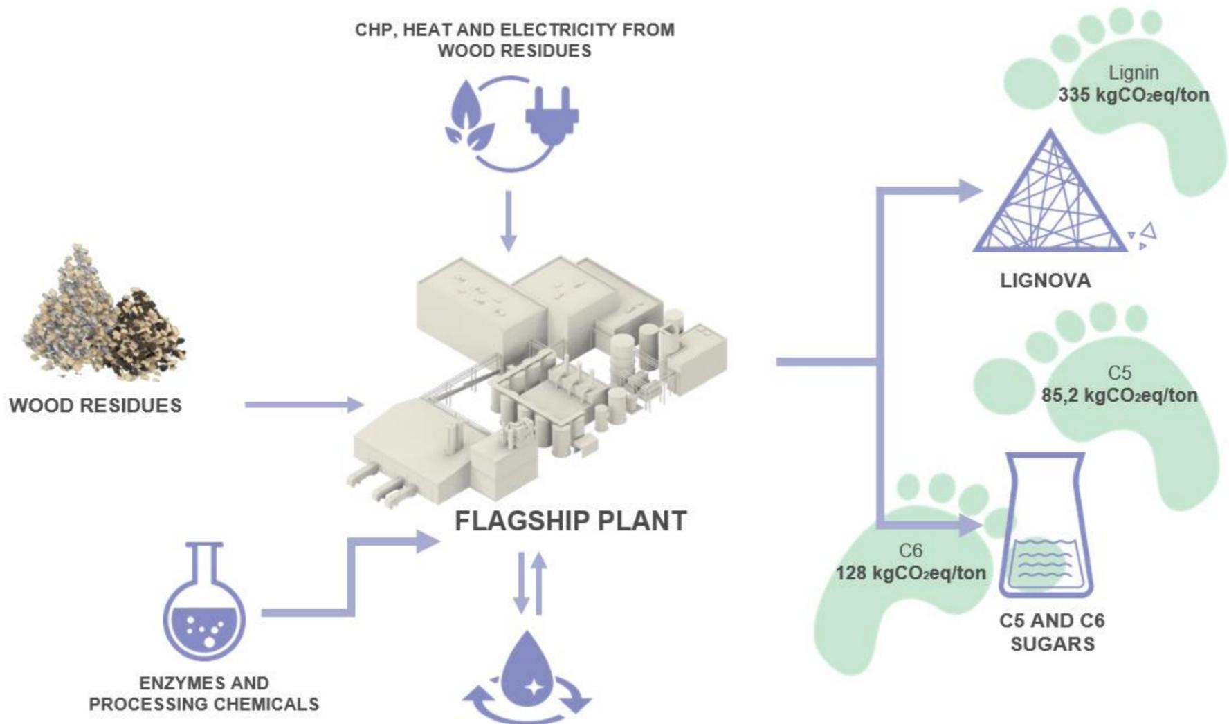
Carbon footprint of lignin, C5 and C6 sugars kg CO<sub>2</sub> per ton final products
