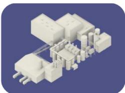
**Fractionation process** – Our flagship plant uses Sweetwater Energy Sunburst pretreatment technology, during which wood is deconstructed into its basic components. The process uses heat, pressure, dilute acid and mechanical power to turn wood chips into a chocolate mousse-like slurry that is further converted into biomaterials. The fractionation process is efficient and fast (taking only 20 seconds to turn wood chips into wood slurry).
